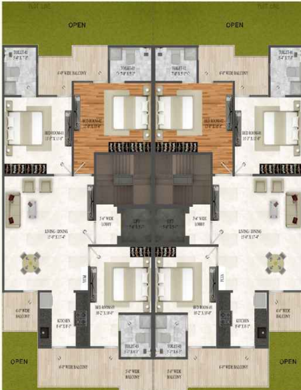
A) Carpet area of the unit: 850 sq. ft. B) Covered area of the unit: 1038 sq. ft. C) Balcony area of the unit: 208 sq. ft. D) Total Built Up Area (B+C): 1246 sq. ft.
