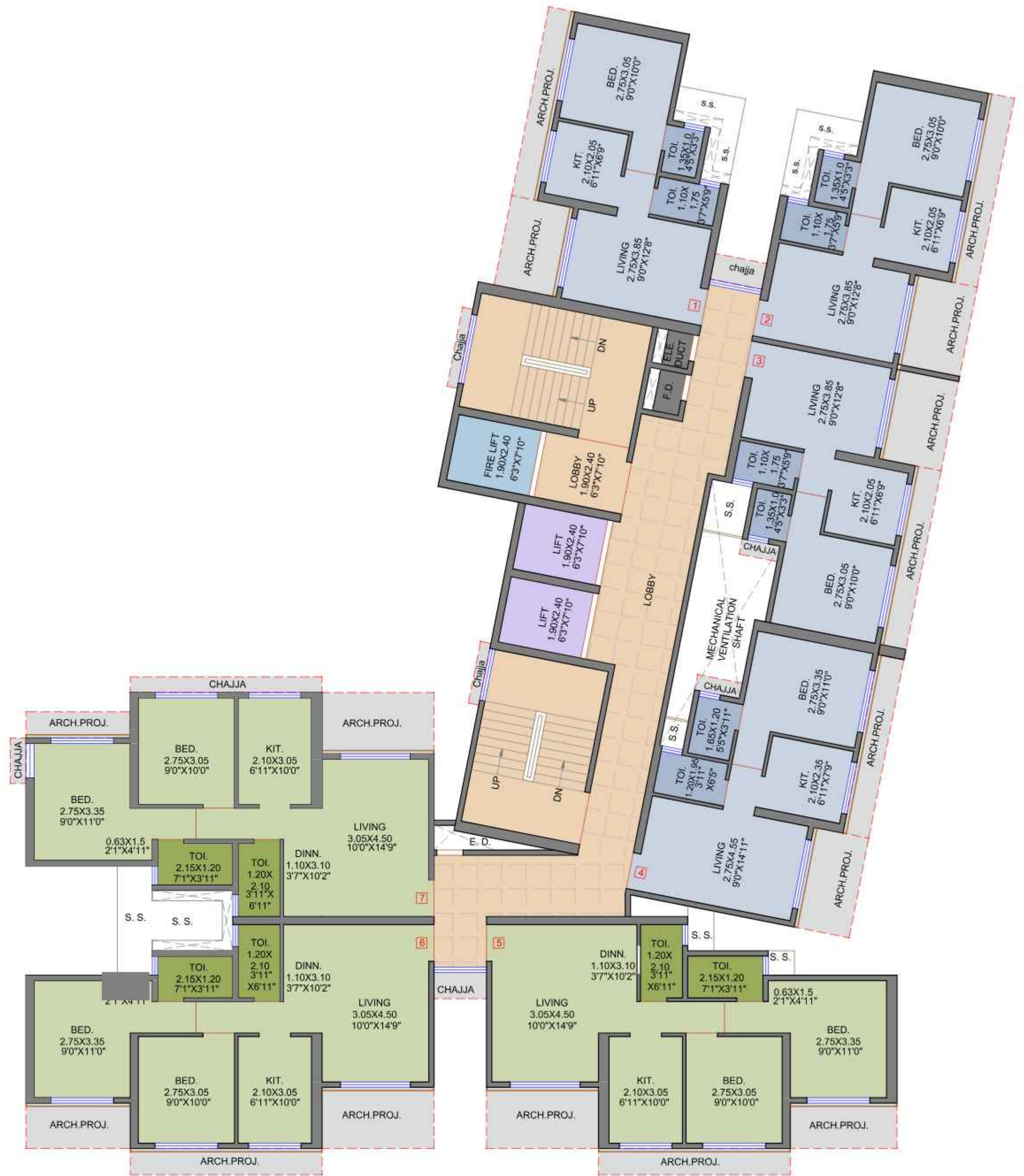
TYPICAL 9TH, 10TH & 12TH FLOOR PLAN SCALE :- 1:100
